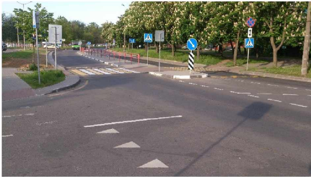
Fig. 3. The typical example of the street-refuge's installation in Minsk, Belarus
