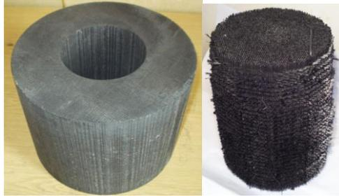
Fig. 1. A model is of ring (after treatment) and cylindrical pre-forms
